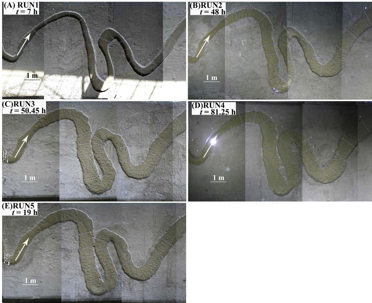
**Fig. 6.** Illustration of the bend evolution in the five experiments. (A and B) Planform of runs 1 and 2 at the 7th and 48th hour respectively; (C and D) the planforms of runs 3–5 at their occurrence of neck cutoff.
