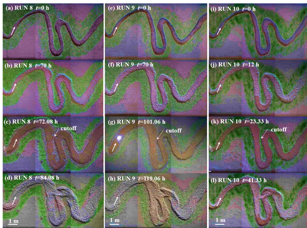
Fig. 5. Temporal changes of bend planform around the neck (bend 3–6) from the initial morphology to cutoff occurrence in RUN 8, 9, and 10.
