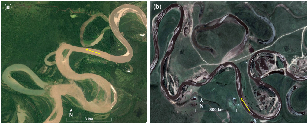
Fig. 3. Two examples showing the co-existence of neck and chute cutoffs within the same section of two meandering rivers with different sizes and physiographic settings. (a) The Ucayali River ( -5.211344^\circ , -74.302247^\circ ). The image was taken on 19 August 2012. The channel width in this segment is between 450 and 790 m. A neck cutoff occurred in the upstream segment, followed by a few chute cutoffs. (b) The Black River, a tributary of the Upper Yellow River, China ( 33.572522^\circ , 102.941661^\circ ). The image was taken on 21 August 2021. The channel width in this segment is between 40 and 50 m. A chute cutoff happened in the upstream segment, while a neck cutoff occurred in the nearby downstream part.
