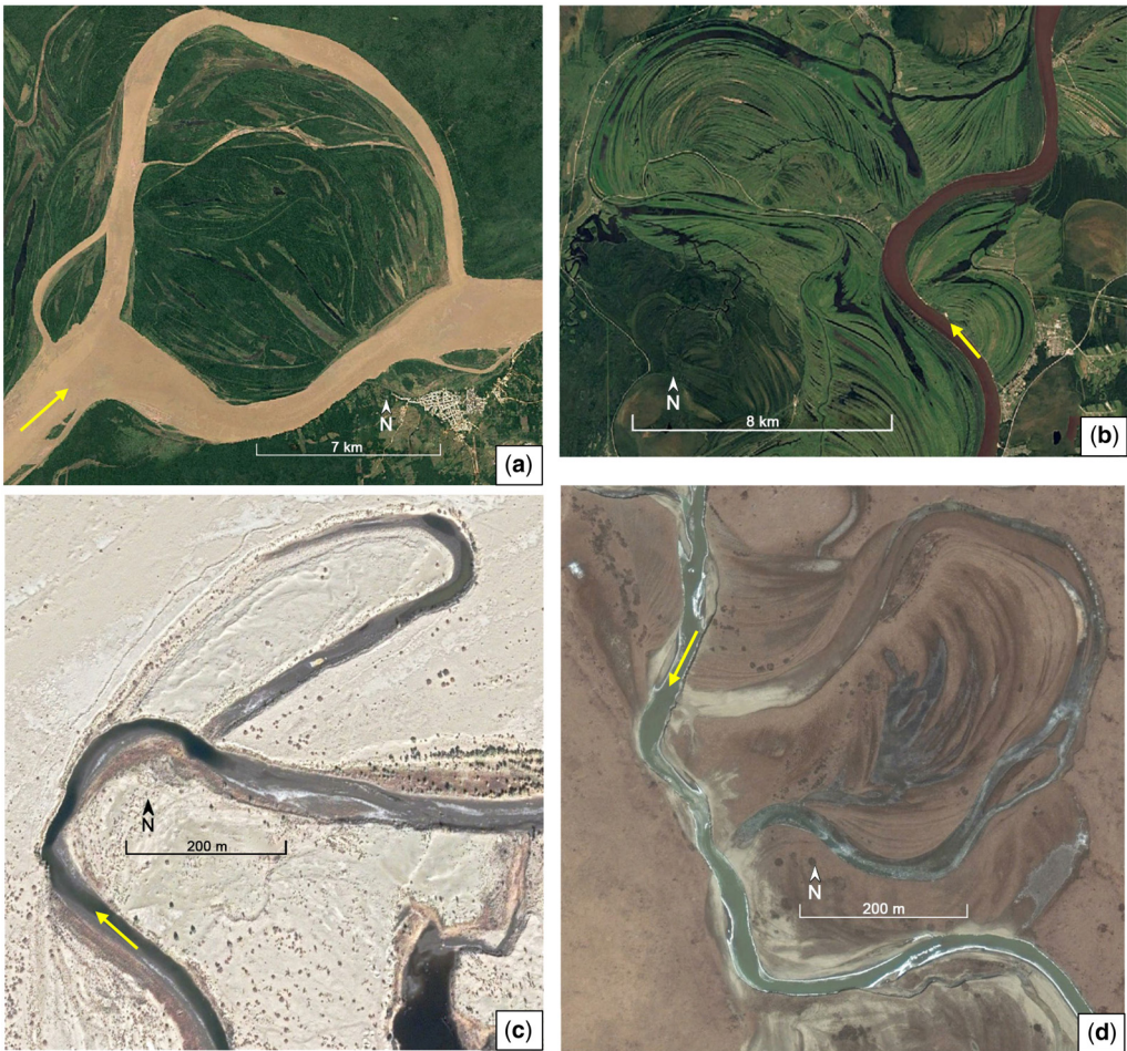
Fig. 12. Meander bends with chute cutoffs by either the mid-channel bar or scroll-sluough mechanisms in different river systems of the world. (a) Amazon River ( -2.513278^{\circ} , -66.146222^{\circ} ). The image was taken in September 2018. (b) The Irtysh River ( 58.456925^{\circ} , 68.286209^{\circ} ). The image was taken in December 2018. (c) The Tarim River ( 40.954539^{\circ} , 87.358348^{\circ} ). The image was taken on 19 October 2019. (d) The Black River ( 33.643548^{\circ} , 103.010519^{\circ} ). The image was taken on 4 December 2014.
